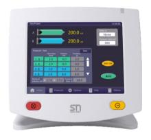
Remote console: able to edit the protocols and execution of injection, synchronous display of all operations of the local console
